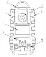
1. Alarm light4. Sensor Port2. LCD Screen5. Button3. Buzzer port6. Buckle
